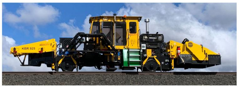
Knox Kershaw's KBR925 Ballast Regulator is a powerful track dressing machine. It comes equipped with a one pass type plow, reversible side wings, and a broom attachment. The machine features a rear mounted engine and a spacious, high visibility cab with unique window placement and hydraulic tilting function. Machine meets or exceeds all FRA requirements. Machine is customizable for converting to multiple gauges ranging from 1435 mm (56.5") to 1676 mm (66").
