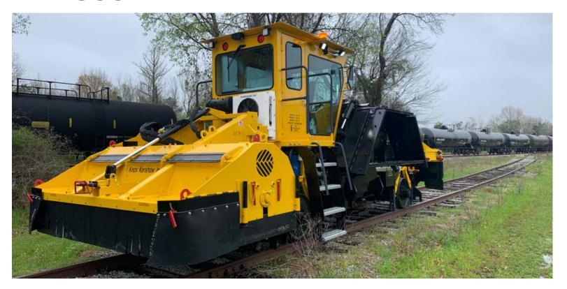
The KBR860 Ballast Regulator is a powerful track dressing machine. It comes standard with a one pass type plow, reversible side wings, and a broom attachment. The machine features a sturdy comfortable cab with unique window placement for optimum visibility. The compact length and short wheelbase are specifically designed to make transport to and from the work site easier.
