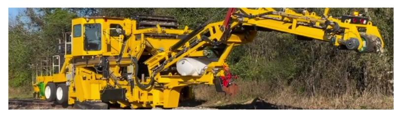
The KYC550 Yard Cleaner clears track and shoulders as well as the space between the tracks on multitrack lines including points and crossings. It is capable of sweeping and loading up to 2.66 cubic yards of waste material per minute. In a single pass the track and fasteners are thoroughly cleared of any unwanted material. The KYC550 is capable of clearing the entire tie width and shoulders for total path width just under 15 feet.
