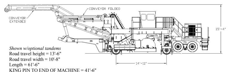
Knox Kershaw's KYC550 Yard Cleaner is designed for cleaning track and switch areas where material is dropped from rail cars.
